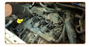
Unscrew the glow plugs. Use a 10 mm glow plug socket. Use a torque wrench. Use a ratchet wrench.
