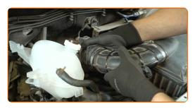
Tighten the clamp that connects the air intake hose to the MAF sensor. Use a 7 mm socket. Use a ratchet wrench.
