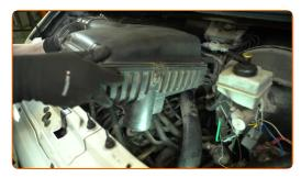
Unscrew the coolant expansion tank fastener. Use a 10 mm socket. Use a ratchet wrench.
