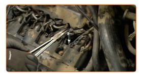
Tighten the glow plugs. Use a 10 mm glow plug socket. Use a torque wrench. Tightening torque: 15 N·m.
