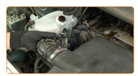
Detach the air intake hose from the MAF sensor.
