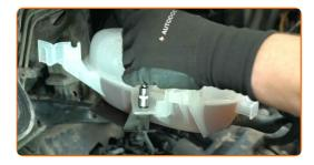
Remove the fastening bolt.
