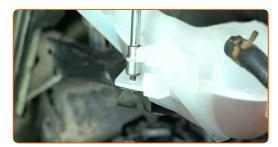
Tighten the expansion tank fastener. Use a 10 mm socket. Use a ratchet wrench.
