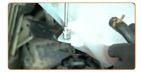
Install the air filter housing together with the air intake hose.
