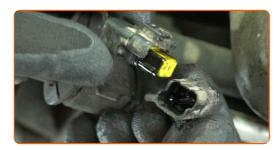
Clean the mounting seat of the crankshaft position sensor. Use an all-purpose cleaning spray.
