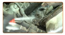
Treat the connector of the crankshaft position sensor. Use an electronic spray.
