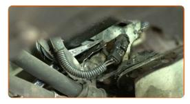
Remove the crankshaft position sensor.
