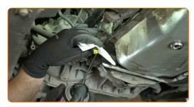
Install the new retaining spring of the crankshaft position sensor.
