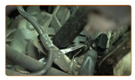
Attach the connector of the crankshaft position sensor.
