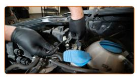
Detach the bulb holder by turning it by ~30°. Remove the holder from the headlight mounting seat.
