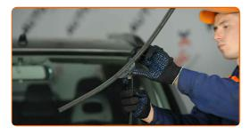
Remove the blade from the wiper arm.
