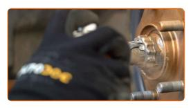
23 Install the brake disc.
