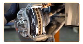
Install the brake caliper and fix it. Use a combination spanner #17. Use a drive socket #14. Use a torque wrench. Tighten it to 26 Nm torque.
