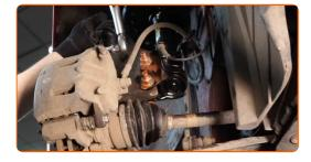
Clean the brake caliper bracket fasteners. Use a wire brush. Use WD-40 spray.
