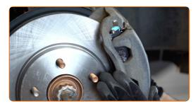
Tighten the brake caliper bracket. Use a drive socket #19. Use a torque wrench. Tighten it to 165 Nm torque.
