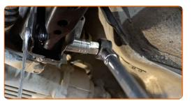
22 Tighten the fastener connecting the stabilizer bar with the control arm. Use a combination spanner #16. Use a drive socket #18. Use a torque wrench. Tighten it to 88 Nm torque.
