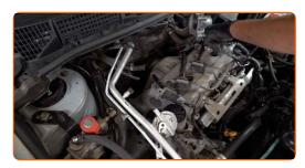
Clean dirt, dust and debris from inside the spark plug well.
