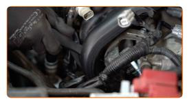
Tighten the fasteners of the intake manifold bracket. Use a drive socket №10. Use a torque wrench. Tighten it to 10 nm torque.
