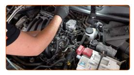
Connect the crankcase ventilation hose to the air duct. Use round-nose pliers.
