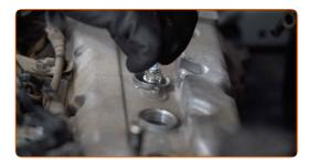
Screw new spark plugs and tighten them. Use the spark plug socket #16. Use a torque wrench. Tighten it to 19.6 nm torque.
