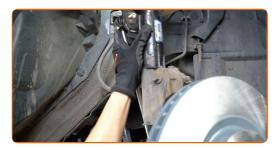
Tighten the fastener connecting the stabilizer link to the stabilizer bar. Use a combination spanner #19. Use a drive socket #19. Use a torque wrench. Tighten it to 65 Nm torque.
