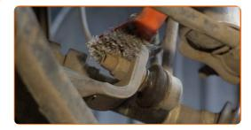
Unscrew the fastener connecting the stabilizer link to the shock strut. Use a drive socket #21. Use a ratchet wrench.
