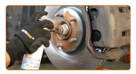
Clean the brake disk surface. Use a brake cleaner.
