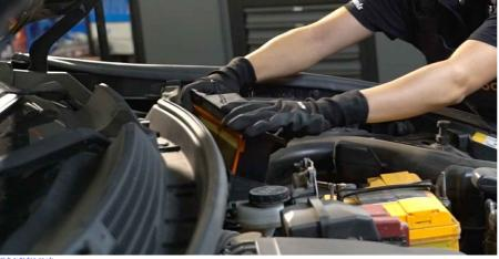
Replacement: air filter – RENAULT KOLEOS (HY\_). AUTODOC experts recommend: Do not apply excessive force when installing the part. Otherwise you may damage the fasteners.
