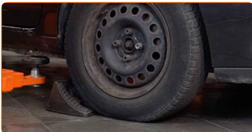
2 Loosen the wheel mounting bolts. Use wheel impact socket #19.
