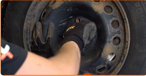
23 Lower the car and working in a cross order, tighten the wheel bolts. Use a torque wrench. Tighten it to 110 nm torque.
