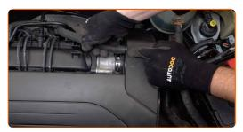
Unscrew the clamp fastening the engine air filter housing to the throttle body. Use a flat screwdriver.
