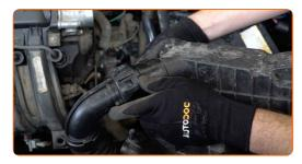
Tighten the clamp fastening the engine air filter housing to the throttle body. Use a flat screwdriver.
