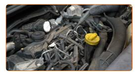
Detach the glow plug wiring connectors.
