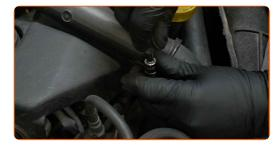
Detach the air intake hose clamp. Use combination pliers. Use a crowbar.
