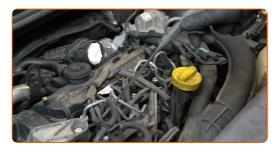
Detach the glow plug wiring connectors.
