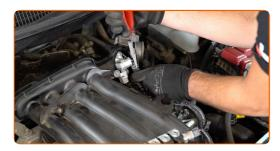
Unscrew the fasteners of the intake manifold bracket. Use a drive socket #10.
