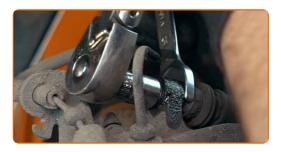
g Remove the brake caliper.
