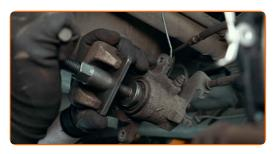
16 Install the brake caliper and fix it.
