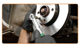
Install the brake caliper together with its bracket.
