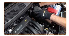
6 Disconnect the crankcase ventilation hose from the intake manifold.
