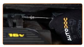
Connect the crankcase ventilation hose to the intake manifold.
