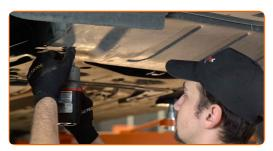
Put a waste oil container with at least 5 l capacity under the drainage hole.
