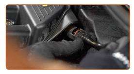
Unscrew the filter housing fastening bolts. Use Torx T25.
