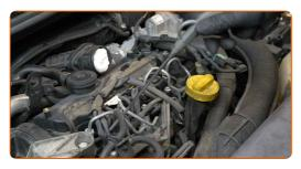
Detach the glow plug wiring connectors.
