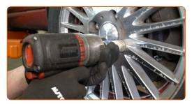
Lower the car and working in a cross order, tighten the wheel bolts. Use wheel impact socket #17. Use a torque wrench. Tighten it to 110 Nm torque.
