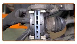
19 Install the brake caliper and fasten it.
