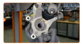
Remove the wheel hub from the steering knuckle. Use a bush and bearing driver set.
