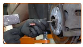
Clean the brake caliper bracket fasteners. Use a wire brush. Use WD-40 spray.
