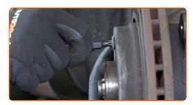
Tighten the brake disc fasteners. Use Torx T40. Use a torque wrench. Tighten it to 10 Nm torque.
