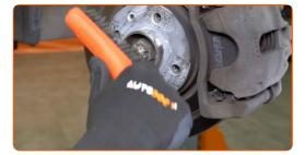
Unscrew the fastener connecting the drive shaft to the wheel hub. Use a drive socket #30. Use a tap wrench.
