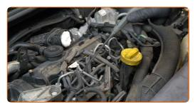
Detach the glow plug wiring connectors.
