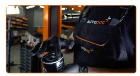
Screw the new filter into its place. Use the 76/14-F socket. Use a torque wrench. Tighten it to 19 nm torque.
