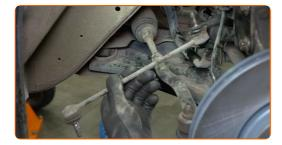
Clean the mounting seats of the stabiliser link. Use a wire brush. Use all-purpose cleaning spray.
