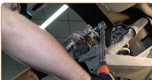
Replacement: wheel bearing – RENAULT Clio III Van (SB\_, SR\_). Tip from AUTODOC:
