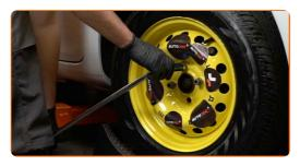
Clean the fastener of the driveshaft. Use WD-40 spray.
