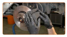
Tighten the brake caliper bracket. Use a drive socket #18. Use a torque wrench. Tighten it to 105 Nm torque.
