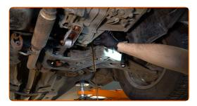
Replacement: manual gearbox oil – RENAULT Clio III Van (SB\_, SR\_).
