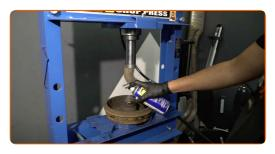
Press fit the new wheel hub bearing into the brake drum. Use a bush and bearing driver set.
