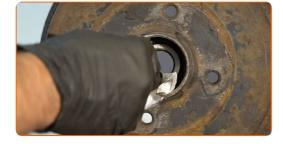
Remove the wheel hub bearing retaining ring. Use circlip pliers.
