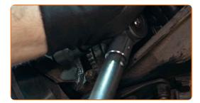
Tighten the fasteners connecting the ball joint to the control arm. Use a drive socket #18. Use a torque wrench. Tighten it to 75 Nm torque.
