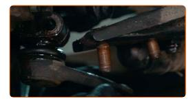
Disconnect the ball joint from the steering knuckle. Use a flat metal-working chisel. Use a hammer.
