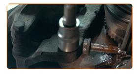
Remove the fastening bolt.
