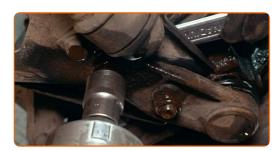
Release the fastener connecting the ball joint to the steering knuckle. Use a crowbar.
