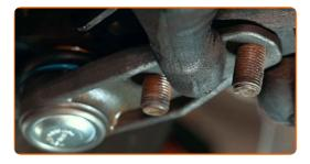
Screw in the fastener connecting the ball joint to the control arm. Use a combination spanner #18. Use a drive socket #18. Use a ratchet wrench.
