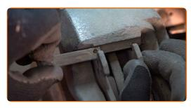
10 Remove the brake pads.
