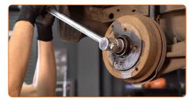
10 Remove the brake drum.
