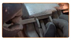
10 Remove the brake pads.
