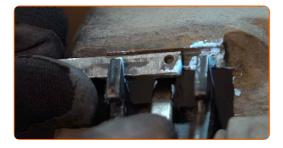
Install the brake pad retaining pin. Use round-nose pliers.
