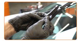
Remove the blade from the wiper arm.
