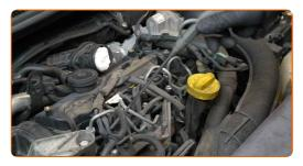
Detach the glow plug wiring connectors.
