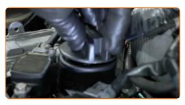
Tighten the oil filler cap.
