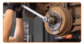
10 Remove the brake drum.
