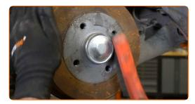
Treat the surface where the wheel rim contacts the brake drum. Use ceramic grease.
