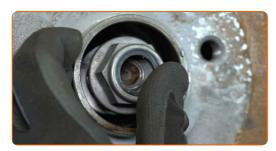
Tighten the hub fastener. Use a drive socket #30. Use a torque wrench. Tighten it to 175 Nm torque.
