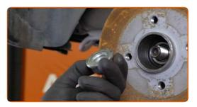
Remove the brake drum assembled with the wheel hub bearing.
