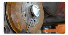
Unscrew the wheel hub fastener. Use a drive socket #30. Use a tap wrench.
