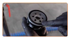
Screw the new filter into its place. Use the 76/14-F socket. Use a torque wrench. Tighten it to 21 nm torque.
