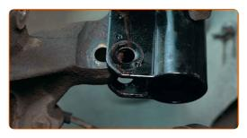
Remove the steering knuckle together with the wheel hub. 29
