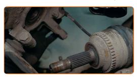
Disconnect the steering knuckle from the shock absorber strut. 28
