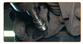
11 Remove the brake caliper together with its bracket.
