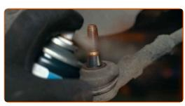
Clean the mounting seats of the tie rod end. Use a wire brush. Use WD-40 spray.
