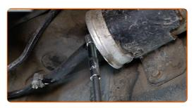
Unscrew the fuel filter bracket. Use a drive socket #10. Use a ratchet wrench.
