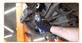
Unscrew the caliper bracket fastening. Use a drive socket #18. Use a ratchet wrench. Use a tap wrench.
