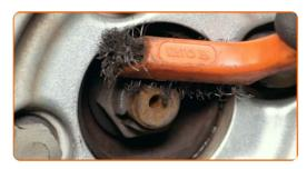
Loosen the fastener of the driveshaft. Use a drive socket #30. Use a tap wrench.
