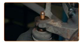
Screw on the fastening nut that connects the tie rod end to the steering knuckle. Use a drive socket #16. Use a tap wrench.
