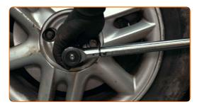
Tighten the wheel bolts using a criss-cross pattern. Use wheel impact socket #19. Use a torque wrench. Tighten it to 90 Nm torque.
