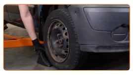
Loosen the wheel mounting bolts. Use wheel impact socket #19.
