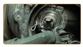
6 Remove the low and high beam bulb.
