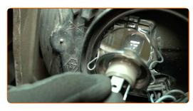
Install a new low and high beam bulb into its mounting seat.
