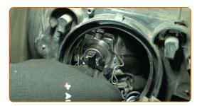
Secure the low and high beam bulb with the retainers.
