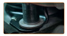
Screw the new engine mount to the bracket. Use a drive socket #16. Use a ratchet wrench.
