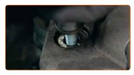
Unscrew the engine mount from the bracket. Use a drive socket #16. Use a ratchet wrench.
