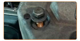
Screw in the fasteners of the engine mount bracket. Use a drive socket #16. Use a ratchet wrench.
